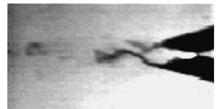
Fig. 4 High-speed image of the metal droplet formation during wire arc spraying. Source: N. Hussary and J. Heberlein, J. Therm. Spray Technol. , Vol 10 (No. 4), 2001, p 2972-2978
